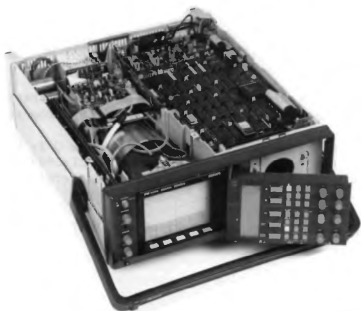
Figure 16.3 Measuring the front unit working condition
